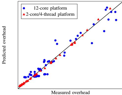
**Fig. 12:** Experimental Vs Predicted overhead for *eAudit*. Predicted values come from the formula for  $O$  in Table 11 and the values of  $t_q$  and  $t_s$  obtained by regression analysis. These values are  $t_q = 2.26 \cdot 10^{-6}$  and  $t_s = 2.06 \cdot 10^{-5}$  on the 2-core platform, and  $t_q = 7.72 \cdot 10^{-7}$  and  $t_s = 2.85 \cdot 10^{-6}$  on the 12-core platform.
