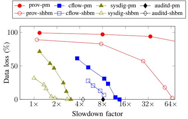
**Fig. 2:** Data Loss: Fraction of events dropped by existing provenance collection systems. The base for calculating the slowdown factor is the benchmark runtime in the absence of provenance collection. The left-most point on each line shows the data loss on unmodified benchmarks. In the legend, “pm” stands for postmark, “prov” for PROVBPF, and “cflow” for CamFlow.
