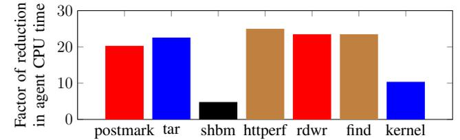
Fig. 17: Performance gains of 2-level buffer design and parameter tuning.
