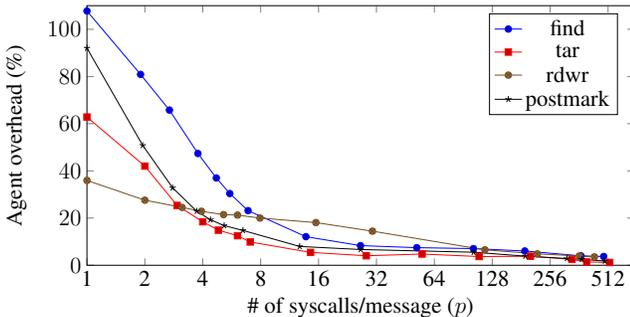
**Fig. 10:** *eAudit*'s Agent Overhead Vs Message Cache Size ( $p$ ). For  $p < 18$ , overhead numbers are an underestimate in cases where there is data loss.
